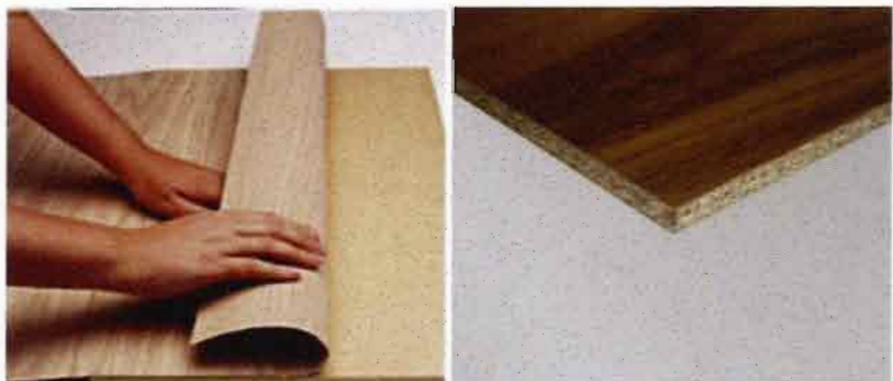
Overlaying wood veneer on a wood panel (left); Particleboard with overlay of wood veneer (right)
