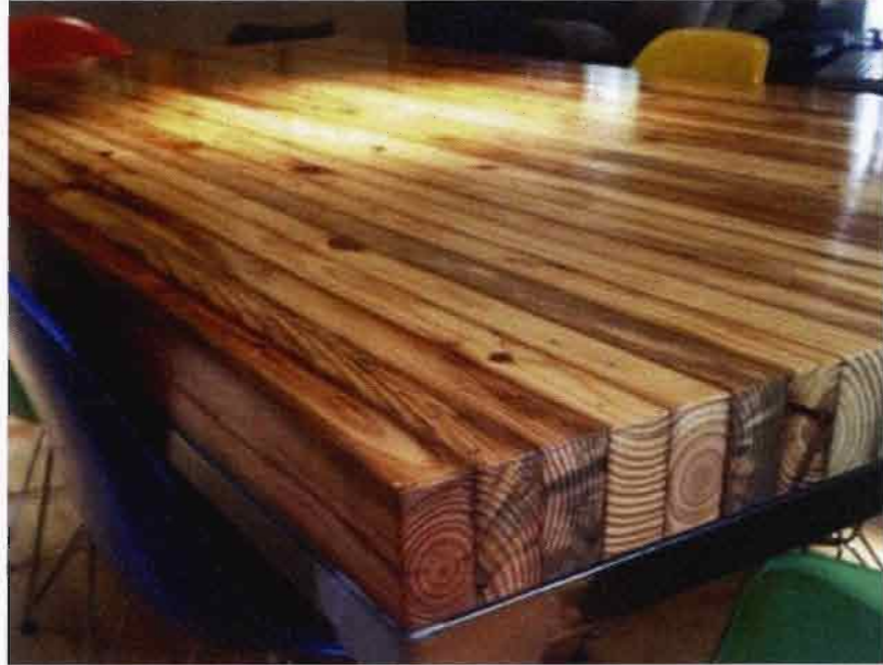
Wooden table top made from side by side lamination of wood pieces
